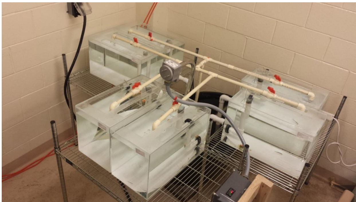
Figure 5. Sump system for testing critical thermal maximum (CTMax) and long-term thermal stress. A pump discharges water into the 37.85-L aquariums and a gravity fed system discharges water into the 189.27-L sump. During CTMax trials, water is heated in the sump by a 5000-W Smartone heater (OEM Heaters, Saint Paul, MN). During long-term thermal stress trials, water is heated in the sump by a 1700-W Smartone heater (OEM Heaters, Saint Paul, MN).
