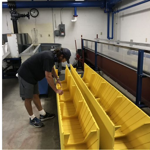
The completed mini Denils are shown in the pictures during a planning meeting for the upcoming study titled "Developing Small-Scale Denil Fishways for Use in Headwater Streams; New Technology and Standards for Increasing the Landscape Connectivity Benefits of Fishways to support Bull Trout, Arctic Grayling, and Cutthroat Trout". (Photo Credit: USFWS-Kevin Kappenman).
