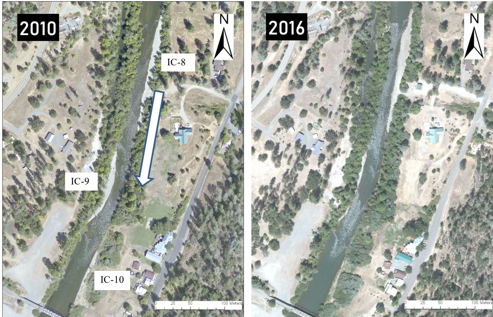
Figure 7. Partial aerial views of Lewiston Cableway rehabilitation site showing a reduction in surface area of three constructed point bars (numbered in left panel) between 2010 at 13.5 (475 ft 3 /s) and 2016 at 12.5 (440 ft 3 /s) m 3 /s, respectively. The white arrow indicates direction of flow.
