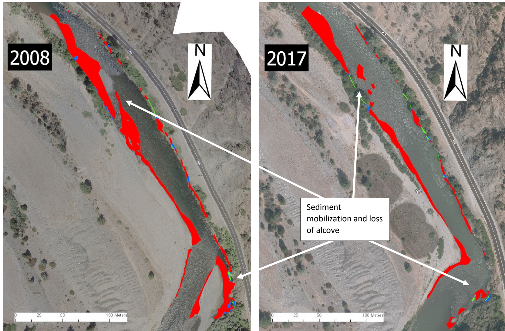
Figure 13. Aerial views of Hocker Flat rehabilitation site showing sediment mobilization and loss of an alcove and medial bar between the post construction (2008) and revisit (2017) surveys. Habitat areas were mapped at 20.3 (717 ft 3 /s) and 15.1 m 3 /s (533 ft 3 /s), respectively. Blue areas indicate optimal presmolt habitat, red and green areas indicate suitable presmolt habitat. The white arrow indicates direction of flow.
