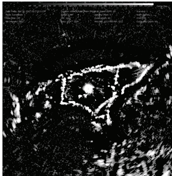
Figure 4. Clutter maps from vertical (left) and horizontal (right) scanning radars at study sites in Ohio and Pennsylvania during the spring 2012 migration season. Brighter areas represent static returns from stationary objects, such as tree lines and fencerows. Target detection may be obscured in these areas because of obstructions from the objects.
