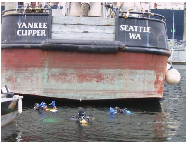
Scientists from the Smithsonian Environmental Research Center prepare to collect images and biological samples of biofouling from a fishing boat. Data are used to determine the effects of season, vessel type, speed, vessel husbandry, and route on the degree of hull fouling.
