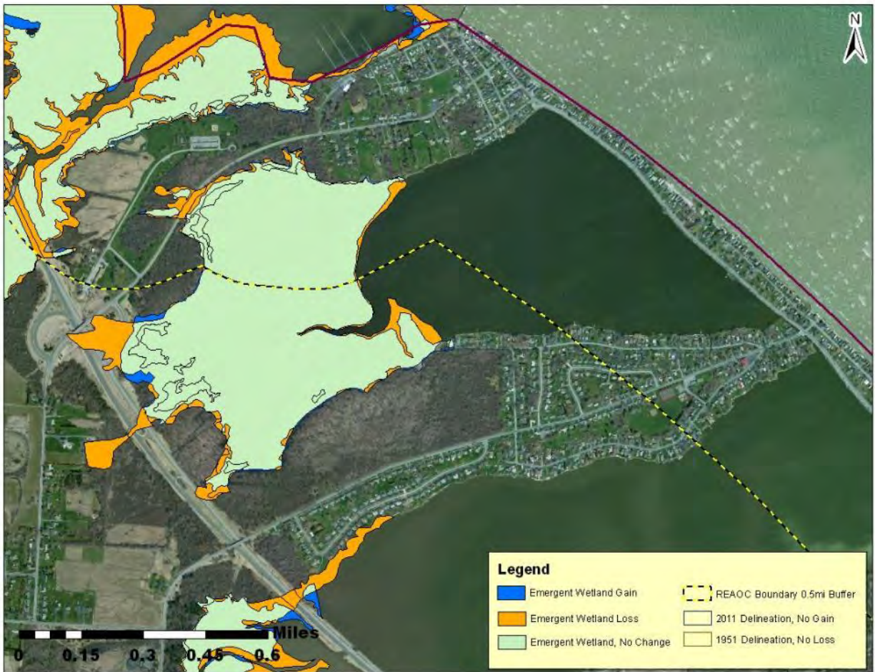
Figure 1-16. Change in wetland extent between 1951 and 2011 associated with Cranberry Pond (center of figure).
