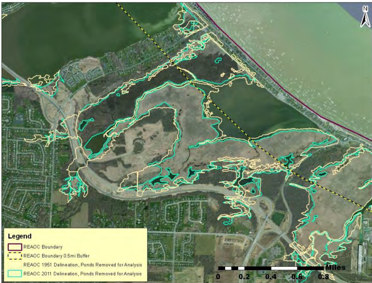
Figure 1-7. Delineated boundaries of emergent wetlands associated with Buck Pond and lower Larkin Creek in 1951 and 2011.
