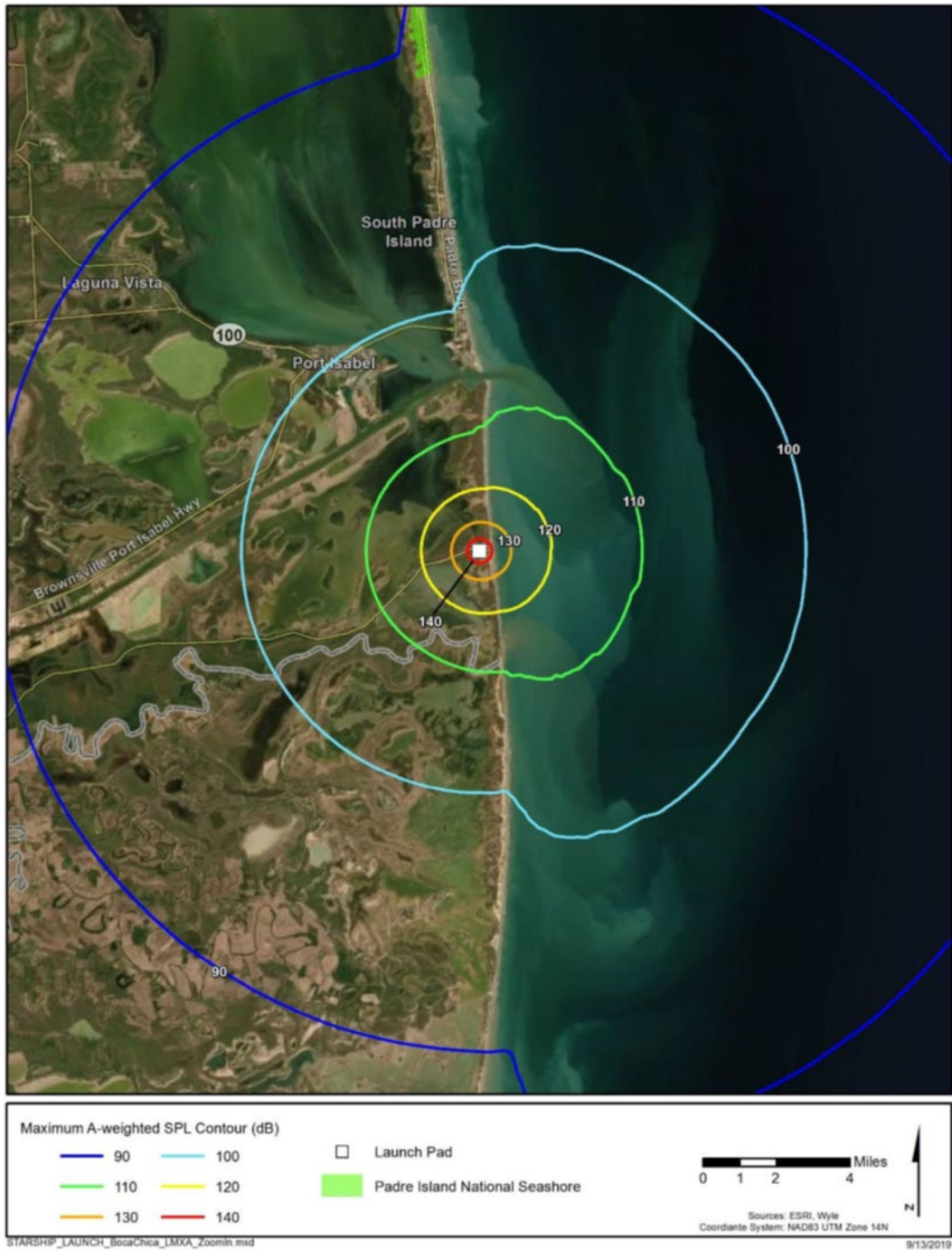
Figure 13. Starship/Super Heavy Launch from the Boca Chica Launch Site: Maximum A-Weighted Sound Levels
