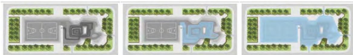
Fig. 28. Top view of the pilot water square - during dry periods, medium rain, and heavy storms (left to right) (© De Urbanisten).
