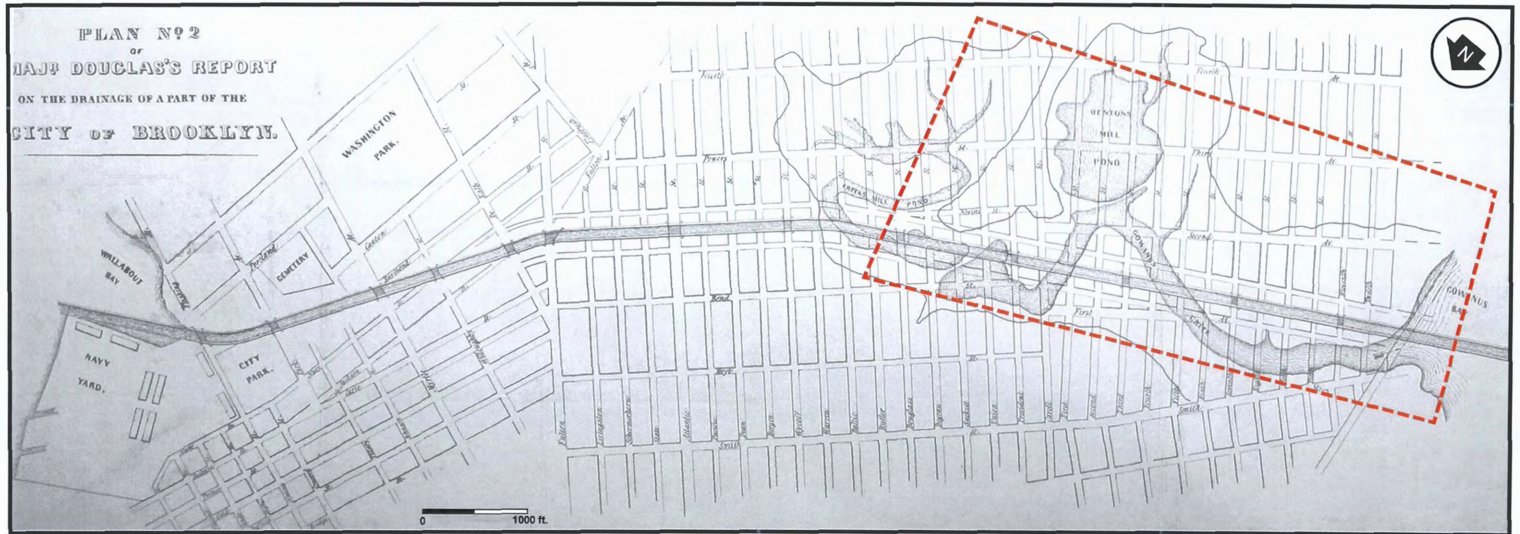
Figure 2.8. Gowanus Canal Assessment of Eligibility: Douglass, Maj. D.B. Plan for Canal from Gowanus to Wallabout Bays. 1870. Scale: 1 inch= 870 feet (approximately). Project area indicated. This is a reprint of the second of Maj. D.B. Douglass' plans for a canal system in Gowanus Creek, including a canal from Wallabout Bay to flush out the Gowanus Creek canal. Dark line around creek and mill ponds is border between marsh areas and slightly higher fast land. Although the Gowanus Canal was not built to this or Douglass' other 1847 plan prepared for the City of Brooklyn, his work presaged the flushing system built in the early twentieth century.
