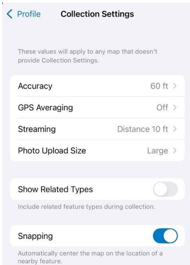
Figure 13. The collection settings tab depicts accuracy, GPS averaging, streaming, photo upload size, related types, and snapping values.
