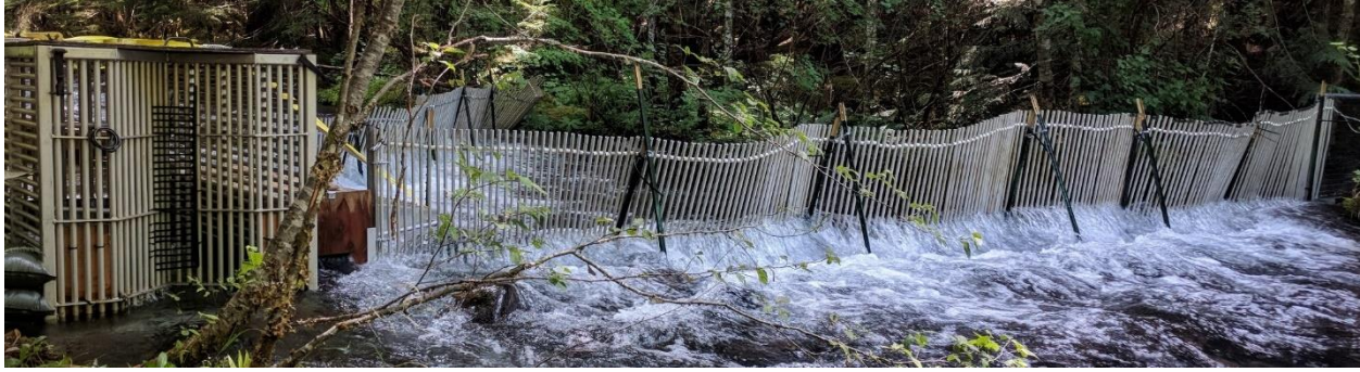
Figure 5. Photo depicting the aluminum picket leads, video chute and trap box deployed in Pinhead Creek.
