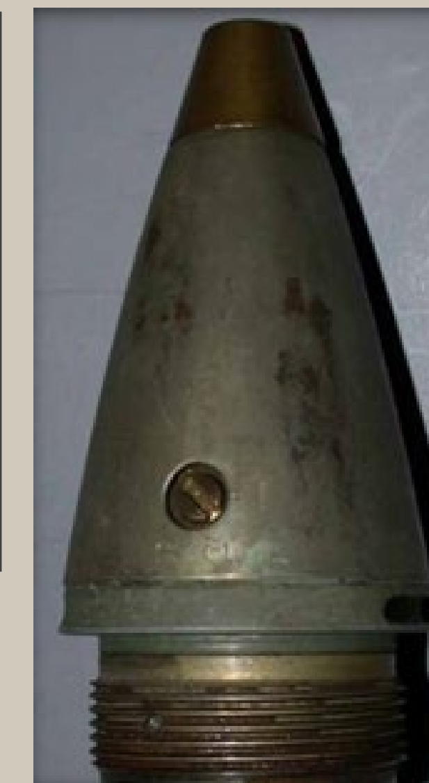
Top Left: M48 projectile fuse with windshield and internal flashtube intact. Top Right: M48 fuse in projectile (no windshield or flashtube). Bottom Right: Fuse cases found decades later on the Refuge.
