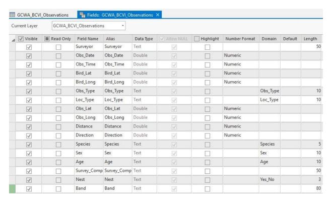
Figure 1. Required GIS Fields for GCWA observation data
