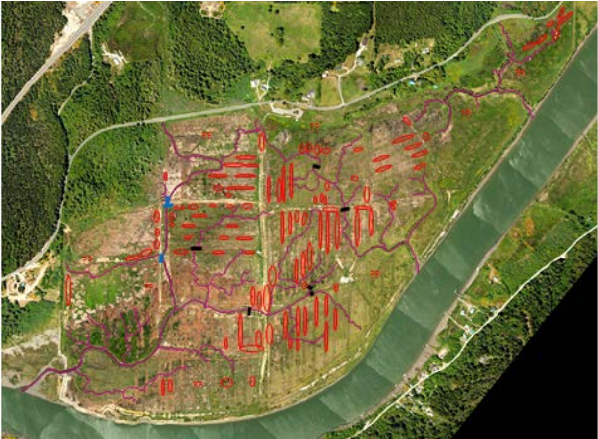
Figure 1. Aerial photograph of the Ni-les'tun Unit with constructed tidal channels indicated in purple. The red ovals surround concentrations of mosquito breeding pools based on 2013 surveys. Black and blue bars indicate footbridges installed to facilitate access.
