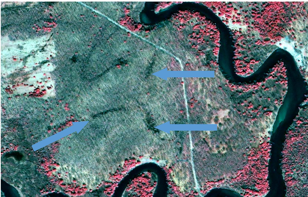
Figure 3 -Early spring 2005 IKONOS satellite image of an area within Michigan. Leaf-off condition makes recognition of wetland features easier. These old oxbows or swales (indicated by blue arrows) can be masked by heavy tree canopy later in the growing season.
