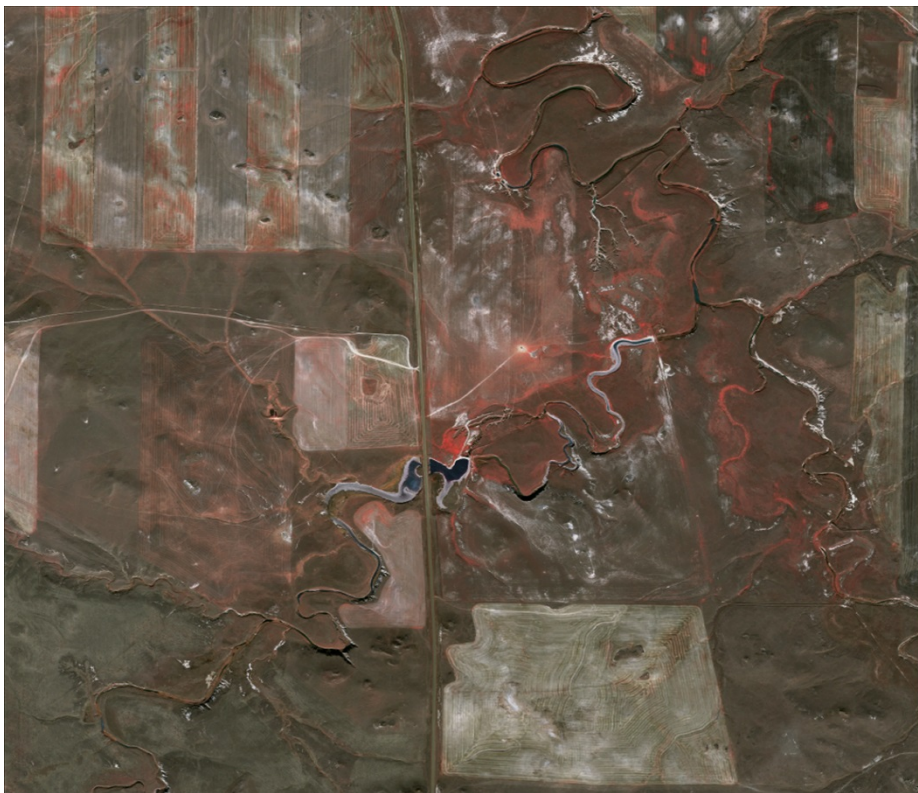
Figure 6 - Fine resolution imagery is the principle data source for determining wetland change. This example shows a false color infrared \leq 1 meter resolution satellite image [GeoEye, 2008].
