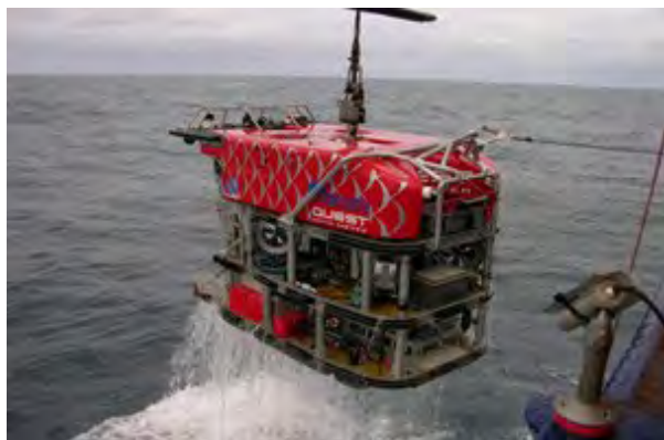
Quest 4000 ROV for deep-sea exploration. Photo: NOAA
