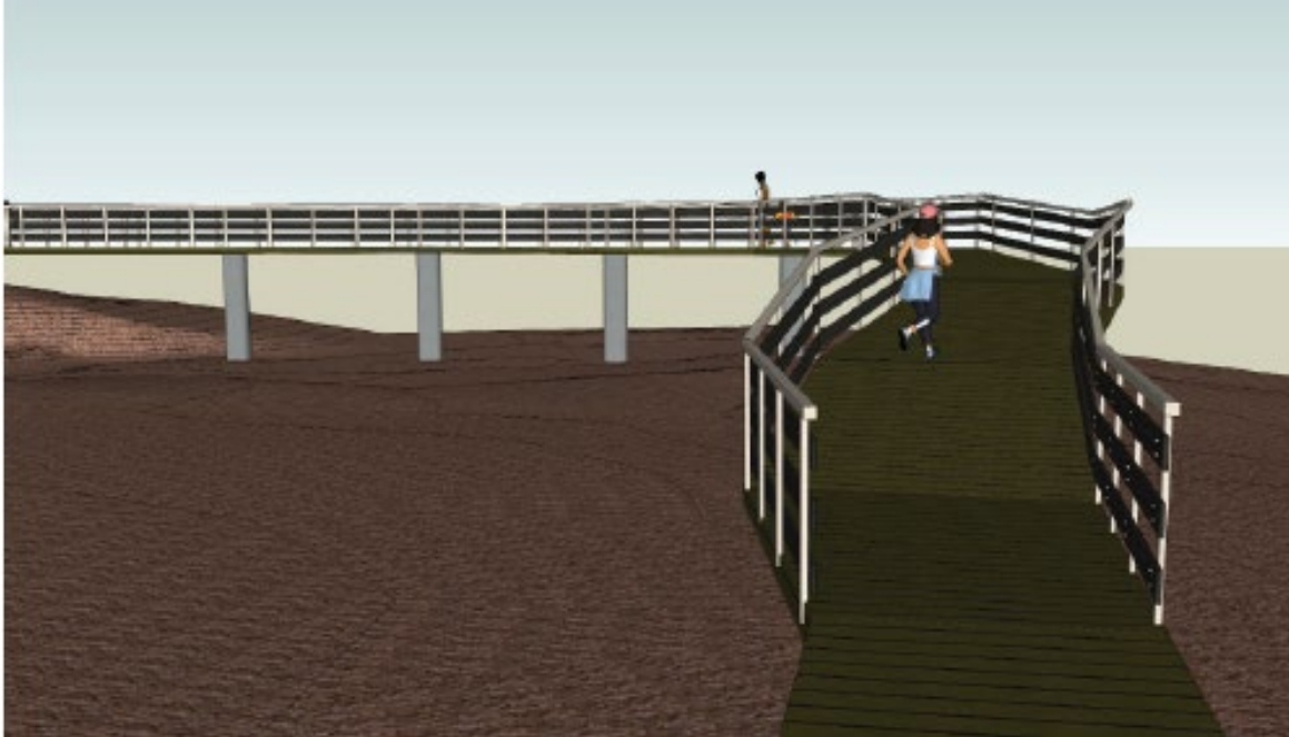
Figure 12. Proposed elevated boardwalk crossing over Steele Canyon Creek, looking north (without trees).
