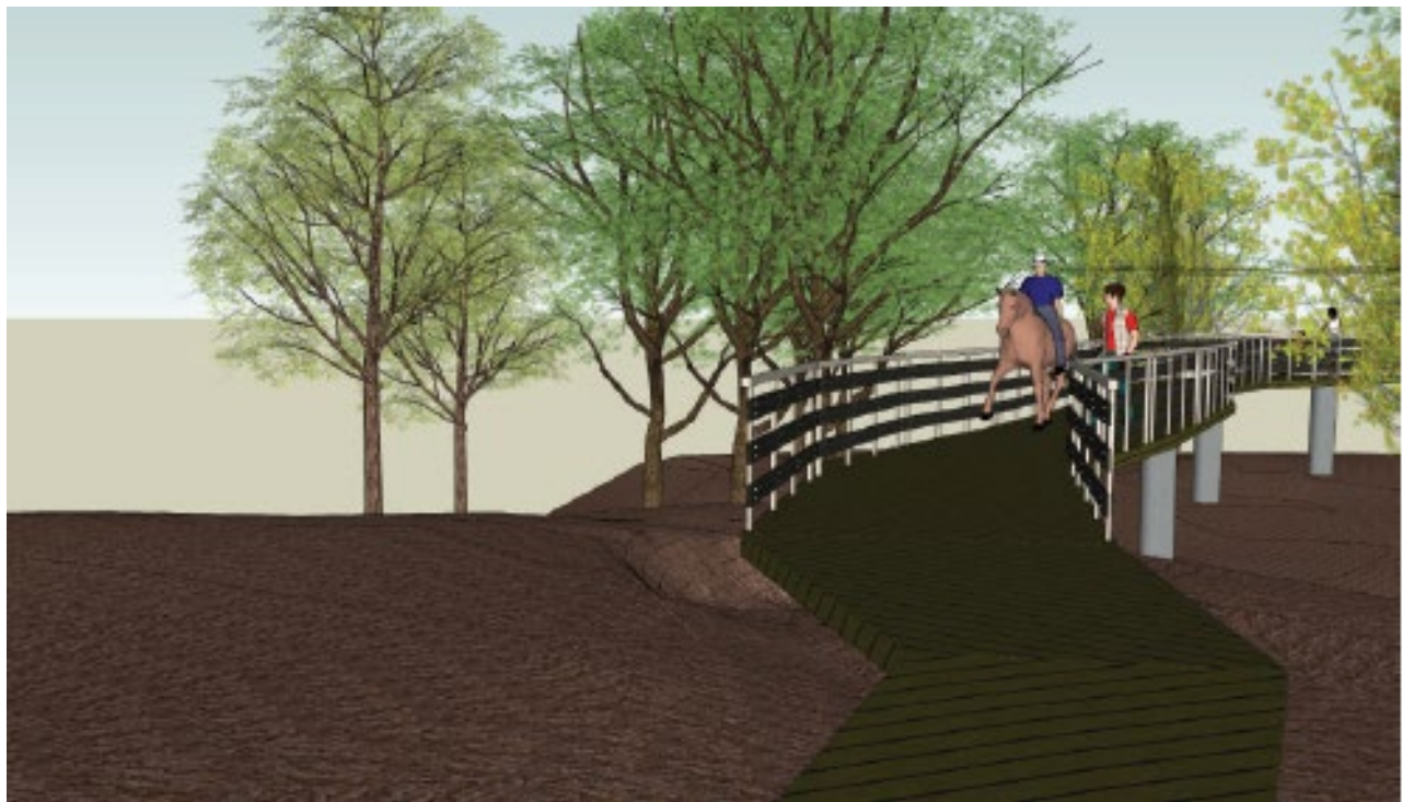
Figure 13. Proposed elevated boardwalk crossing over Steele Canyon Creek, looking south (with trees).
