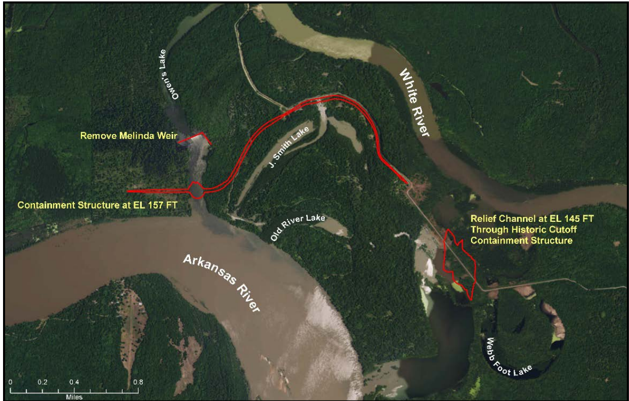
Figure 15: Alternative 1 Containment Structure Alignment
