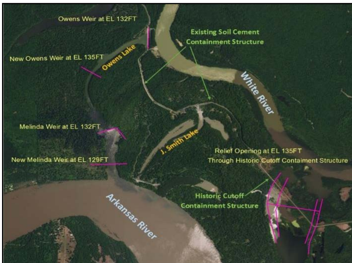
Figure 16: Alternative 2 Containment Structure Alignment
