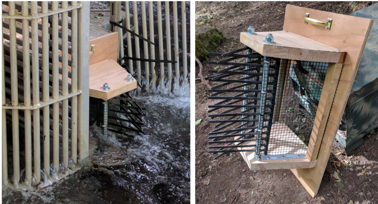
Figure 4. Exclusion gate for video chute.
