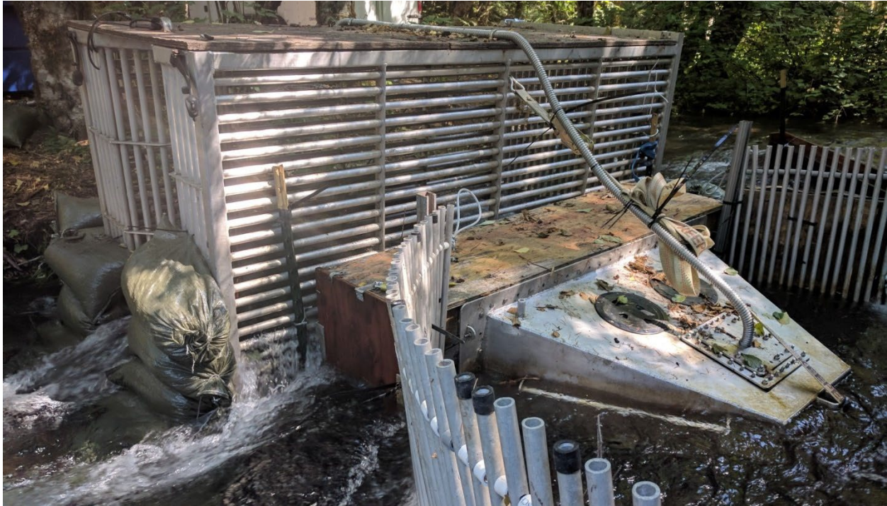
Figure 6. Photo depicting the camera chamber (right), video chute (middle) and trap box (left).
