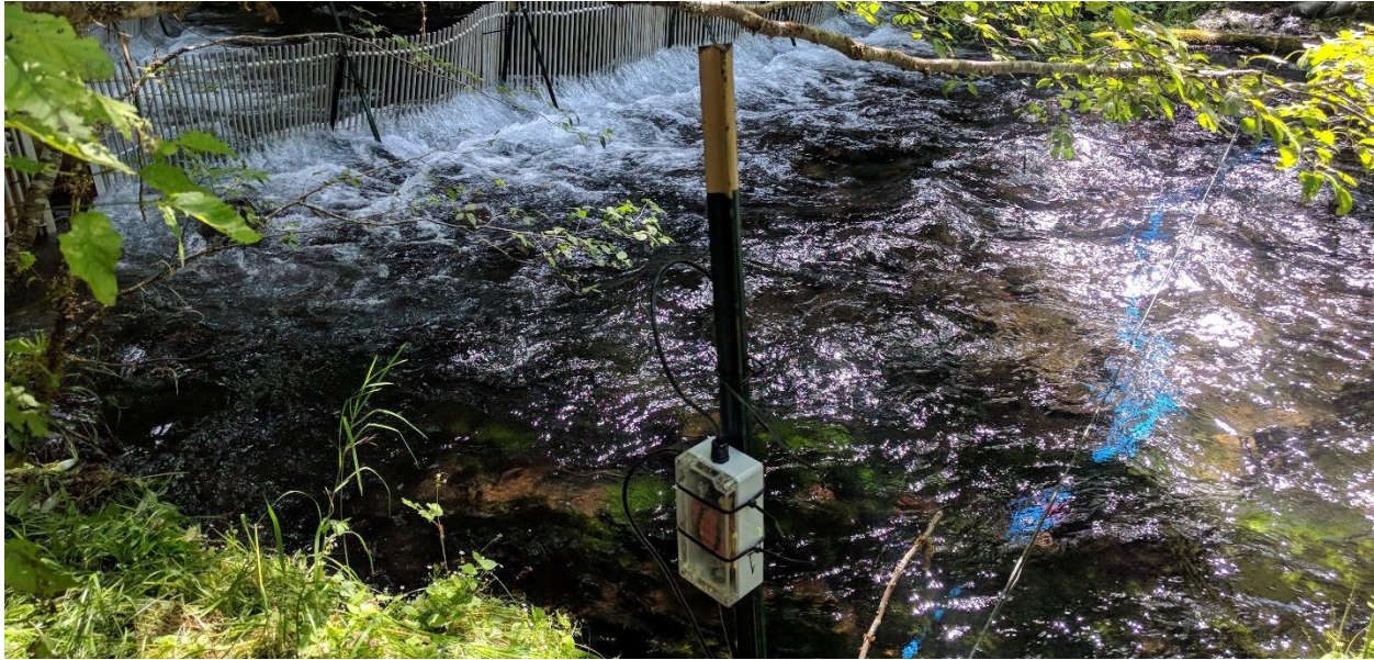
Figure 7. Channel-spanning HDX PIT tag antenna located 150 meters upstream from the Pinhead-Clackamas confluence, approximately 10 m below the Pinhead Creek weir.
