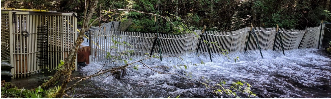
Figure 5. Photo depicting the aluminum picket leads, video chute and trap box deployed in Pinhead Creek.
