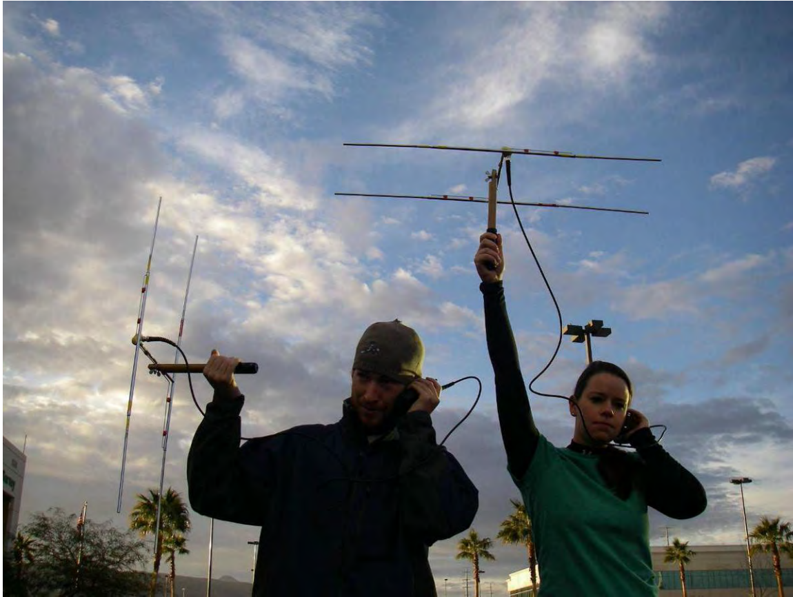
Figure 4. The Vertical antenna position on the left (handle parallel to the ground) provides more range but less directionality in detecting the signal, while the Horizontal antenna position on the right (handle perpendicular to the ground) allows better directionality while lessening range.
