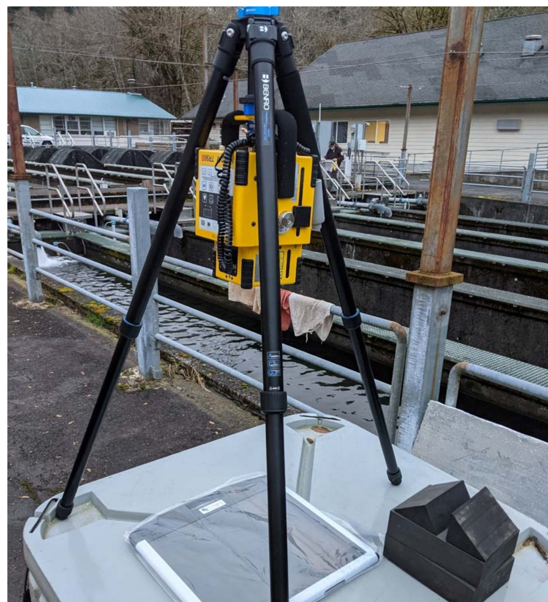
An x-ray system showing the generator and the DR panel which sends images wirelessly to a laptop. Photo credit: Doug Peterson/USFWS
