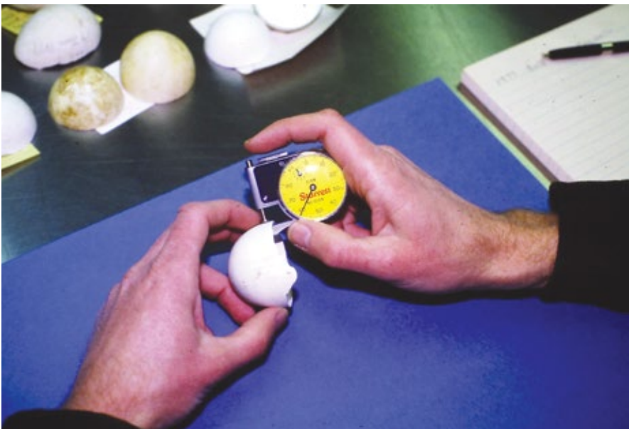
Researcher measuring the thickness of an eggshell with a micrometer to document eggshell thinning by DDT. USFWS
