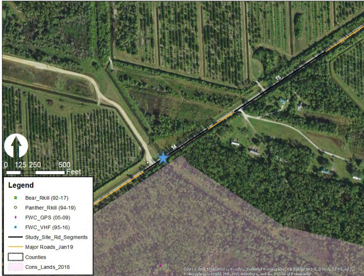
Figure 26. Identified wildlife crossing points at road segment nos. 14 and 15 on Corkscrew Road. Road segment no. 14 includes a large culvert for a canal that crosses under Corkscrew Road. This canal continues north to SR 82 where FDOT is constructing ledges under the road for wildlife passage. The blue star indicates the location of the existing culvert for the canal.
