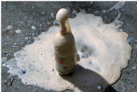
Figure 16: Adding certain mint candies to a bottle of soda causes very impressive bubble formation. The reason is that the crystal structure on the surface of the candy carries millions of microbubbles. When the candy goes into the freshly-opened soda, the very high TDGP of carbon dioxide causes gas to surge into those microbubbles and expand them producing big quantities of foam.
