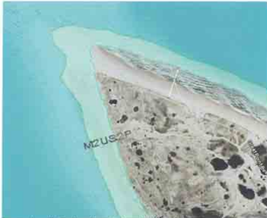
Figure 3: Land boundary shift of nearly 70 meters indicated by white line
