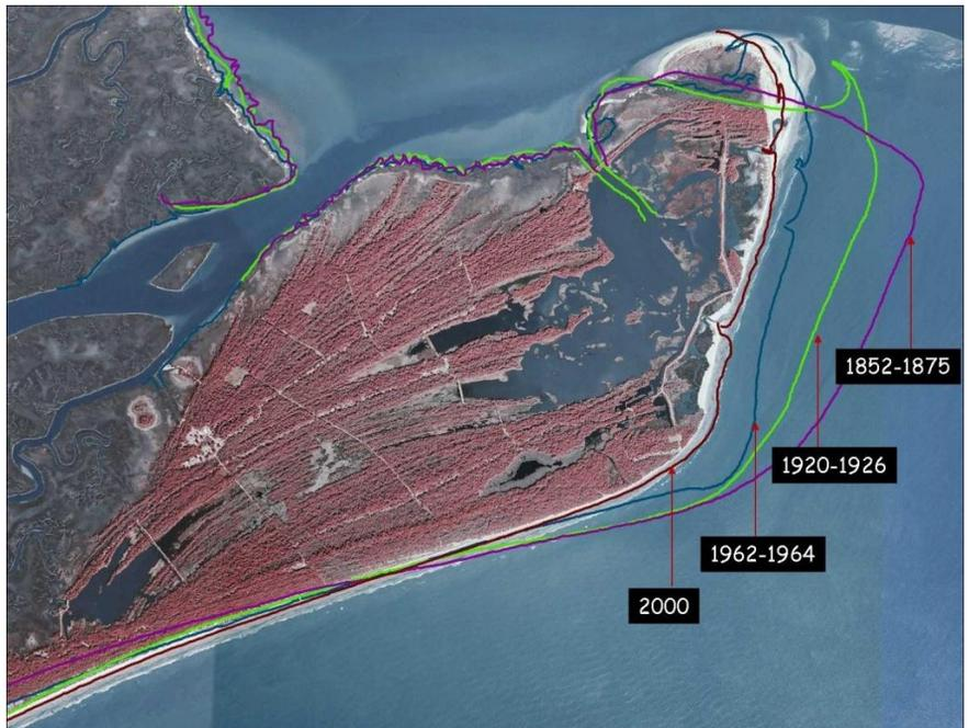
Historical shoreline of Bulls Island shows severe erosion since 1852. The current rate of erosion is approximately 20 feet per year.
