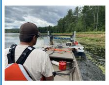
The US Fish and Wildlife Service worked with First Light Power in Turners Falls, MA, to manage a patch of water chestnut in their generation canal. Staff used a specially designed piece of equipment we call *The Conte Cutter* to mulch water chestnut, leaving it unable to produce viable seeds for reproduction.
