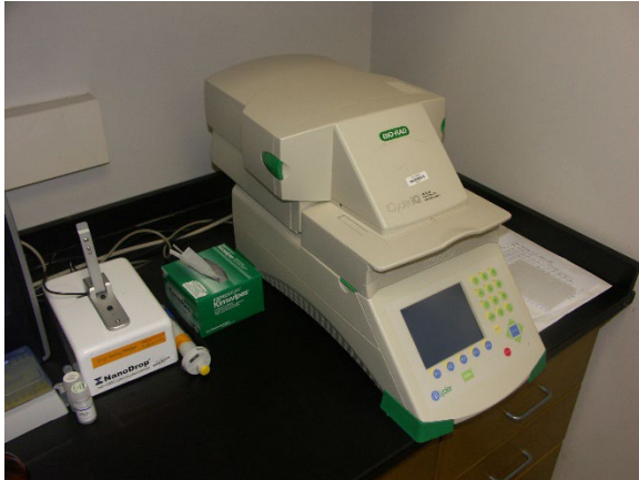
Figure 5: This PCR machine can make billions of copies of pathogen DNA sequences in 96 samples in just over an hour.
