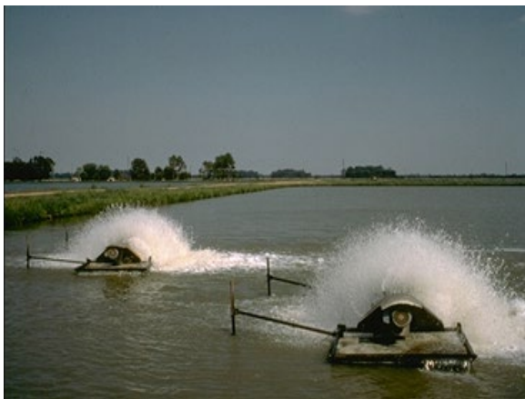
Figure 30: Paddlewheel aerators preventing the formation of an algal scum that catfish could feed on.
