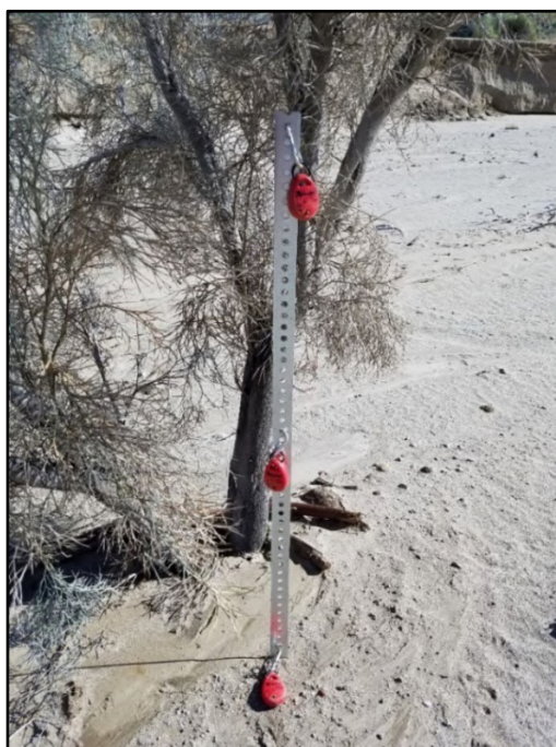
Figure 7. Temperature data loggers (Kestrel Drop D1®) attached to an aluminum stake prior to underground installation to record soil temperature variation at a long-term survey plot. 6
