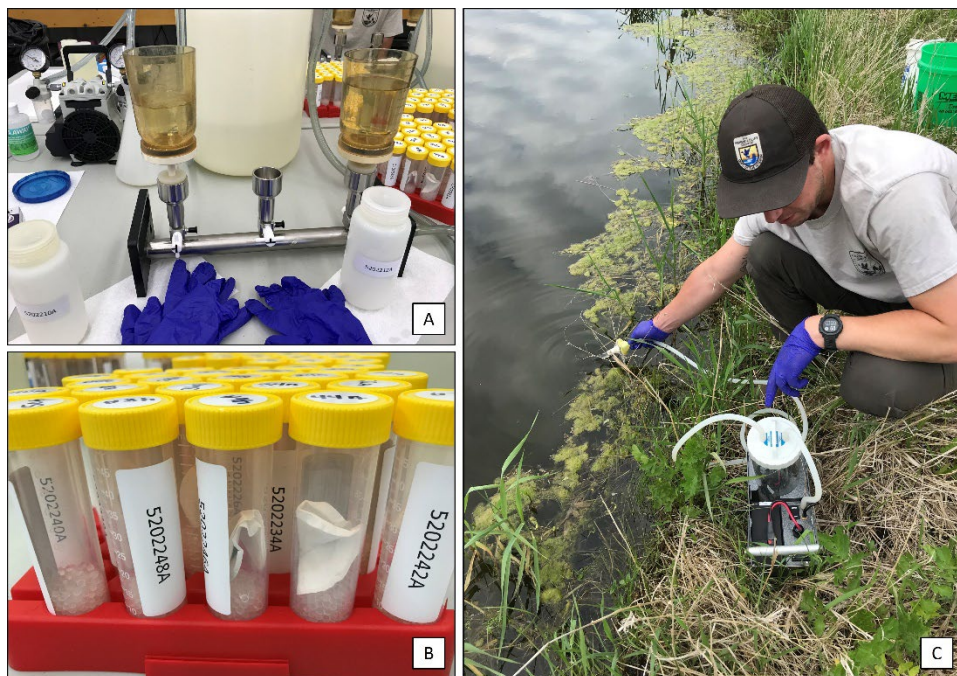
Figure 4. A) Vacuum manifold filtration apparatus used to filter surface water grab samples; B) Completed filters placed in tubes with desiccant beads; C) Water sample collection and filtration in the field using Smith Root Citizen Science Sampler and filter packs.
