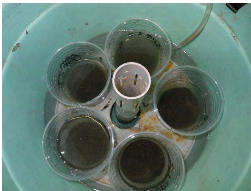
Figure 22. Sediment burrowing time experiment, with individual ammocoetes in each exposure container.
