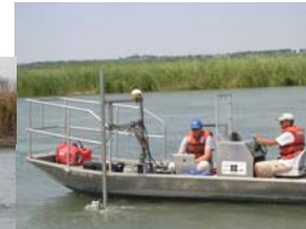
Researchers mapping habitats at pallid sturgeon collection locations with an hydro-acoustic Doppler profiler.
