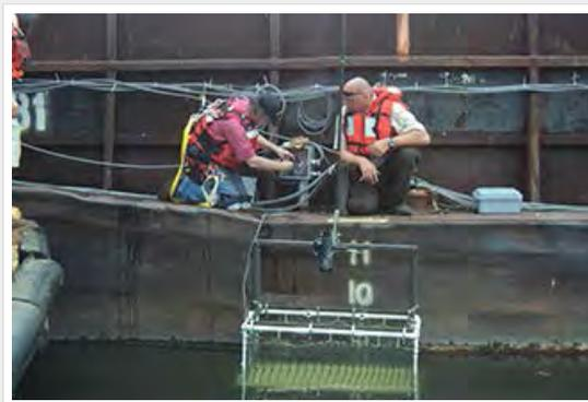
USFWS biologist Aaron Parker (right) helps rig video equipment to a barge set to pull caged fish through the barrier. Credit: USFWS
