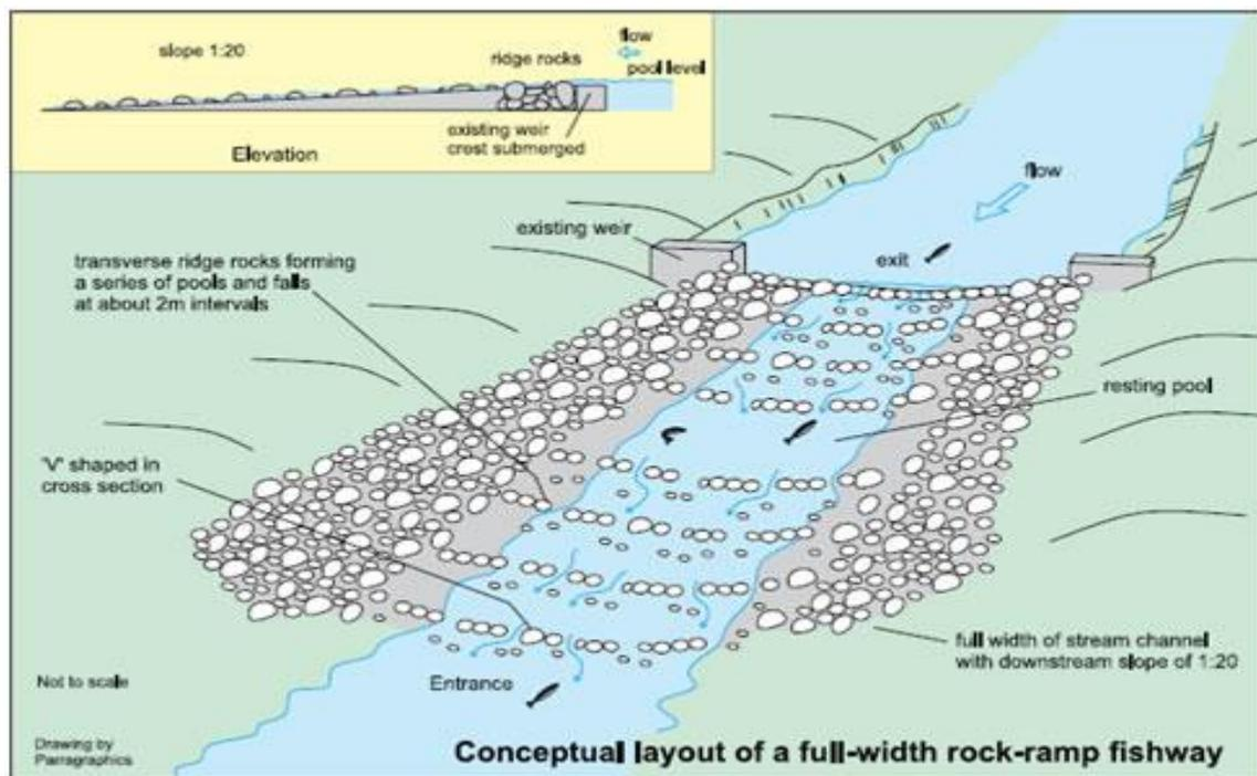
This figure (from the Corps of Engineers) is included to show the concept of a full-channel rock ramp. The specific dimensions do not pertain to this project.
