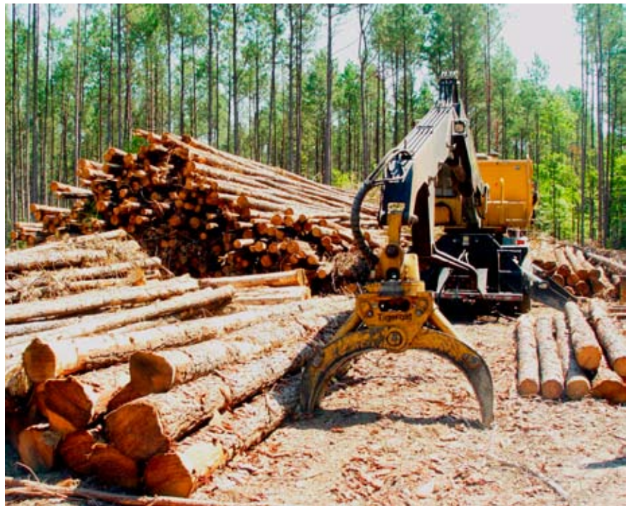
Pulp wood piles, pole timber, and chip logs surround a Tiger Cat knuckle boom loader during thinning work at James River National Wildlife Refuge in Virginia. Gerald Vickers, USFWS
