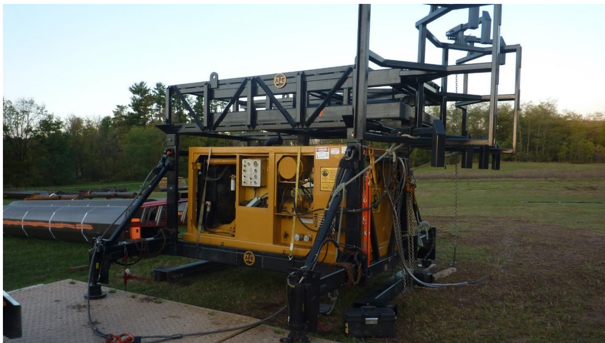
Figure 4 Generator and pile guide
