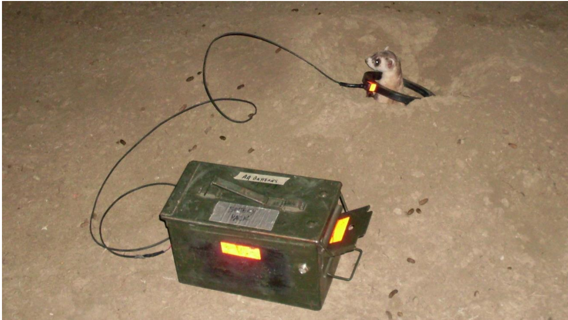
Figure 29. Black-footed ferret passing through a ring reader in Saskatchewan, Canada. The reader is configured for long-term field deployment with a sturdy case and batteries that can last for 2 weeks. Photo by Travis Livieri.
