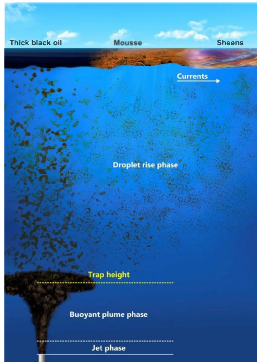
Figure 12. Conceptual depiction of rising plume and trap layer (from French-McKay, 2015).
