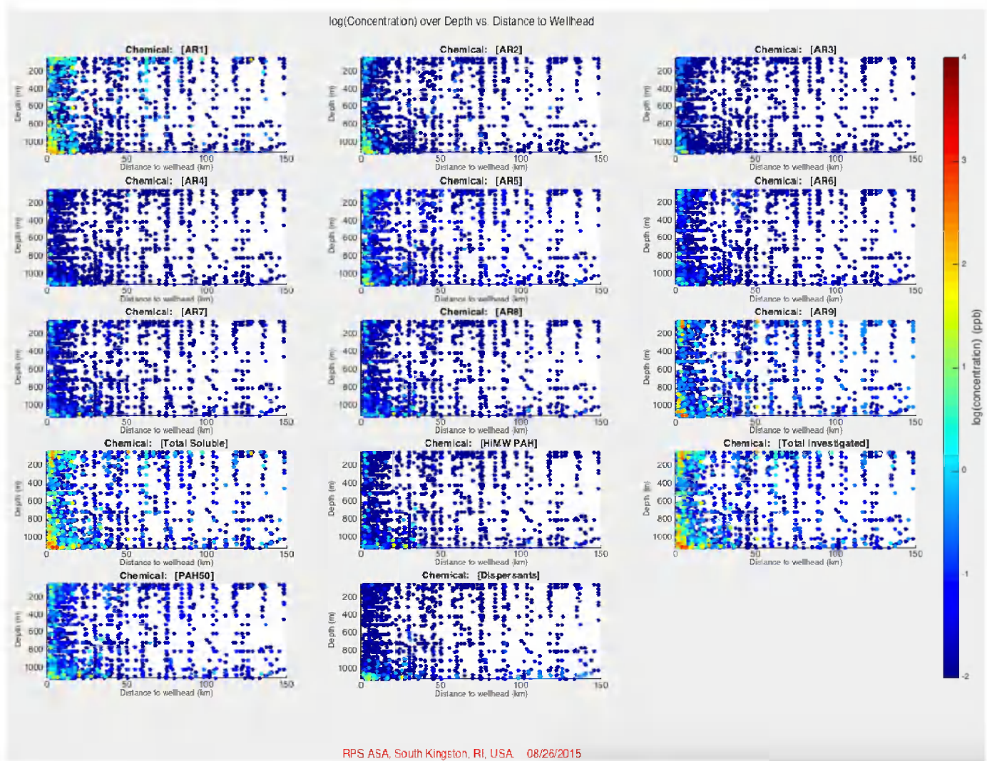
Figure E.2-9. Observed chemical concentrations ( \mu\text{g/L} , or ppb) by grouping on a log-10 scale (color) through the water column (40-1100 m – vertical axis) as a function of distance from the wellhead (0-150 km – horizontal axis). Note that all points represent significant hydrocarbon/dispersant concentrations, above the method detection limit for each investigated compound.
