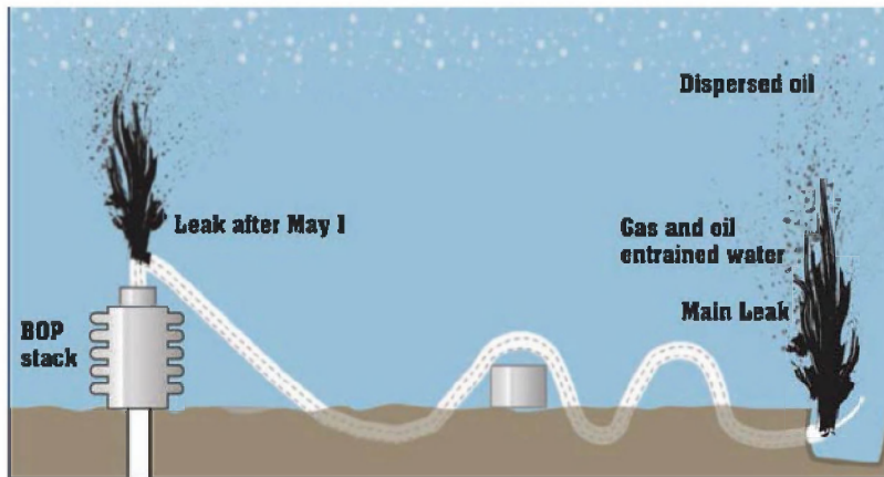
Figure 4-4. Schematic of releases of oil and gas from the end of the riser pipe and from small holes at a kink in the riser pipe above the BOP (Lehr et al. 2010).
