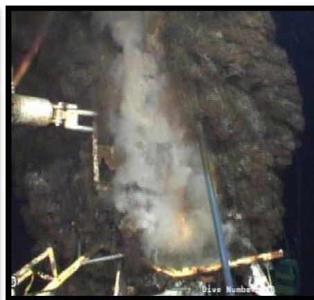
Figure 5-12. Photographs from the ROV video of the wand (upper) and trident (lower left and right) dispersant application methods. Wand dispersant application method (upper). Trident application method (lower left and right).
