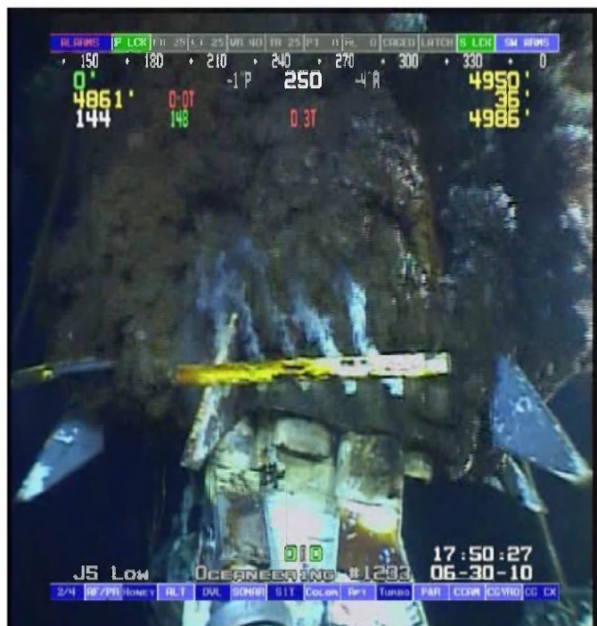
Figure F-10: Flow of oil around the rim of the top hat from ROV images on June 30, 2010.
