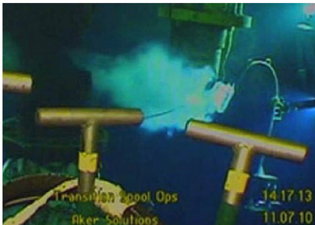
Figure 5-14. A sketch of the hooked wand for dispersant application (left) and an image (captured by Millennium22 on 7/11/10 at 14:17), showing its temporary application (right).
