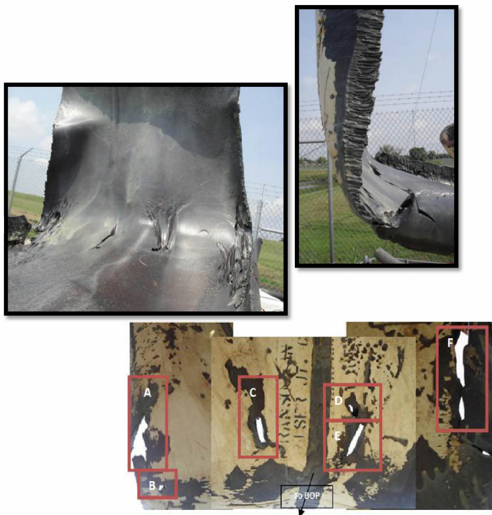
Figure 5-10. Photographs of the kink location, inside to outside (upper left), side (upper right) and outside to inside, (lower center) views taken at the NASA Michoud facility. (Photos taken by Andrew Bird, May 2012.) The holes are identified as A, B, C, D, E, and F (lower center).
