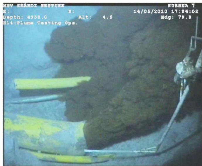
Figure F-8: Release from the end of the riser pipe on May 14, 2010 from the Skandi Neptune . The dispersant wand is noted at the lower right of the image.
