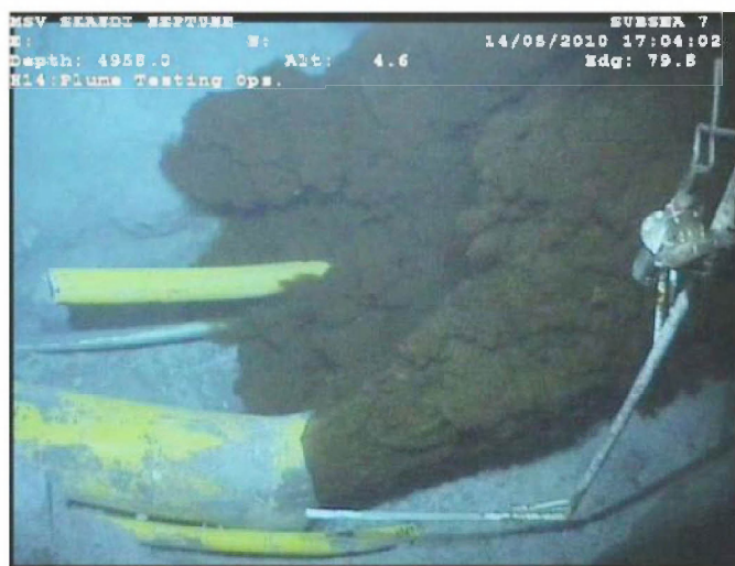
Figure 5-6. ROV image of the end of the riser pipe taken by MSV Skansi Neptune on May 14, 2010.
