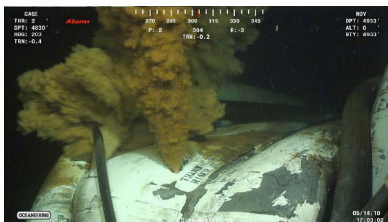
Figure 5-7. ROV image of the kink above the BOP taken by Maxx3 May 14, 2010 (Round 1, Packet E).
