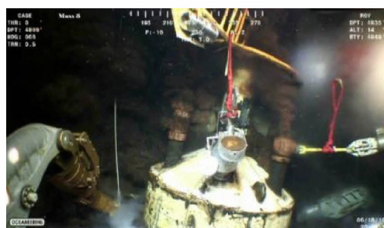
Figure 5-13. Image captured by Maxx3, June 18, 20:06:13 (Round 1, Packet K - DVD 98). The top of this picture indicates the presence of a dispersant ring (or a collar), but it seems that no dispersant is being applied at the specific moment when the image has been captured.
