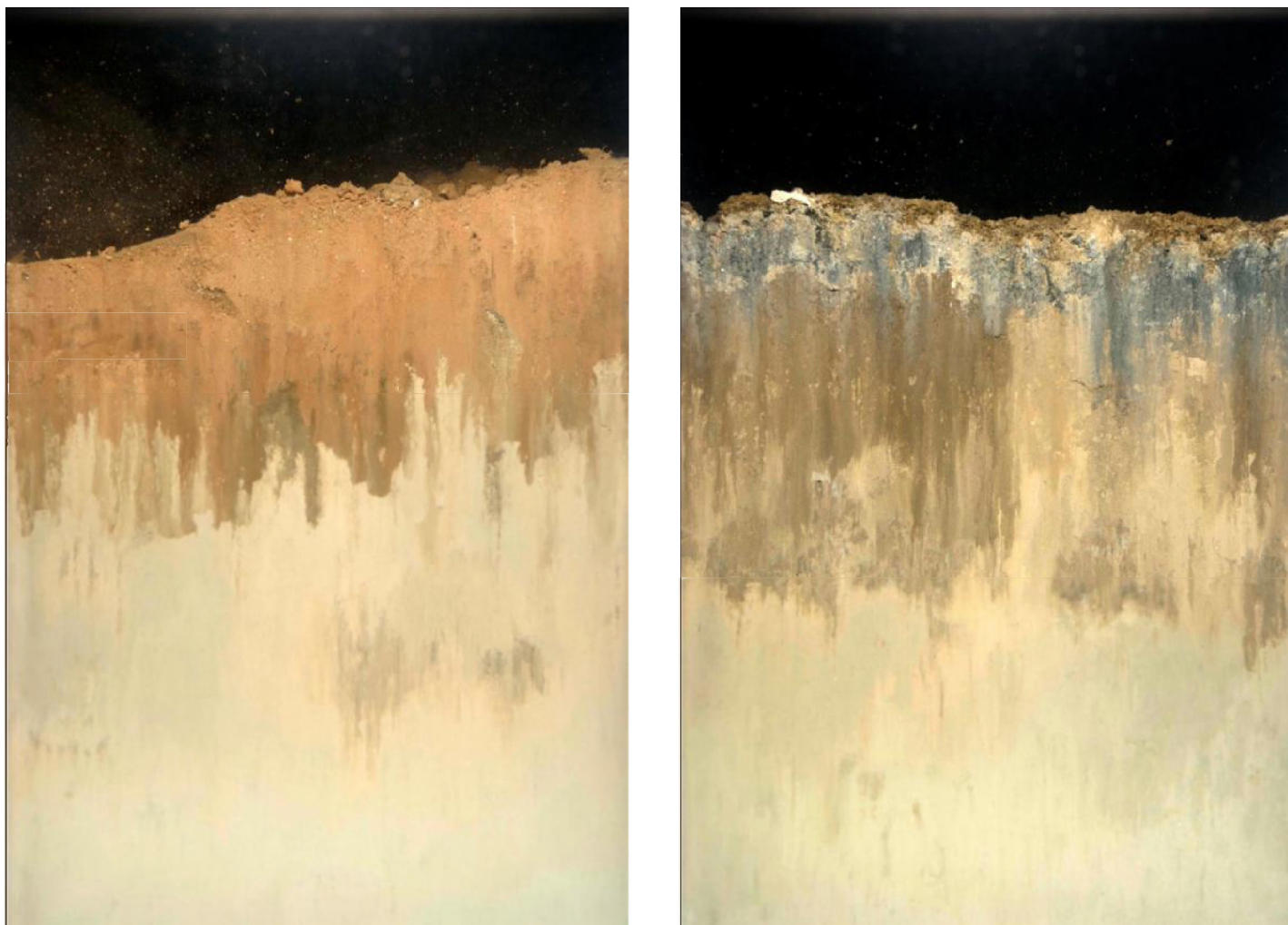
Figure 32 Decrease in aRPD depth moving toward the wellhead along transect 180 from Station 180-5200 (Left) to Station 180-300 (Right)
