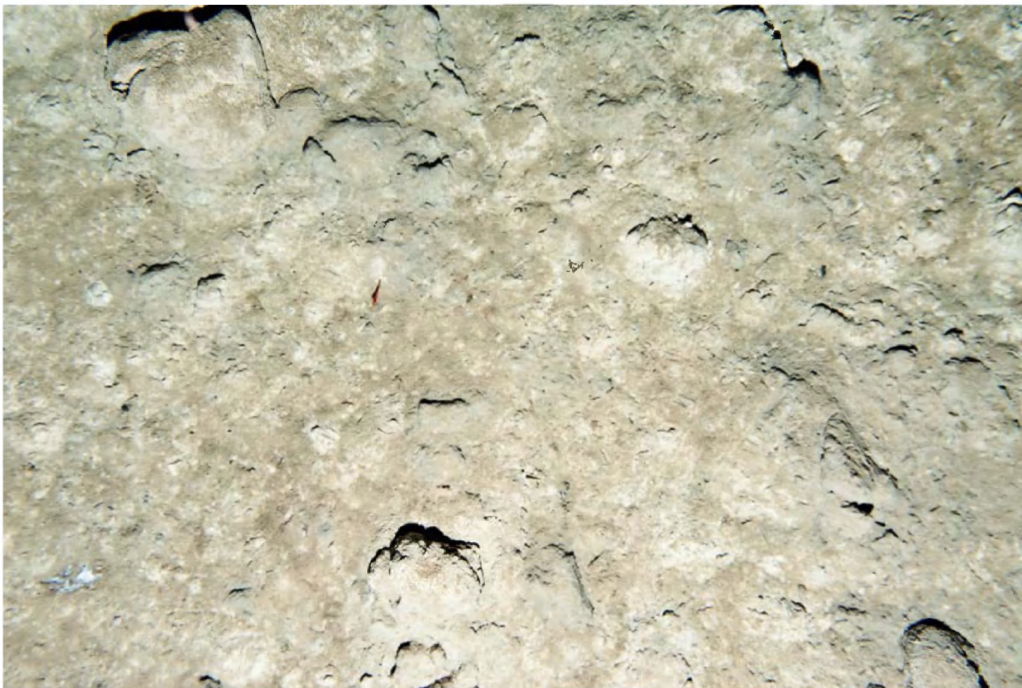
Figure 21 Irregular Surface Texture of Redeposited Pleistocene Muds from Top Hole Drilling shown in PV Image from Station D038-SW
