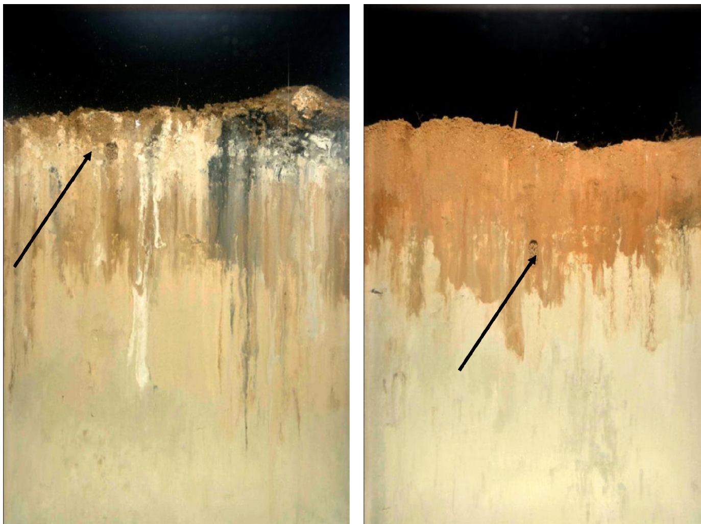
Figure 38 Evidence (arrows) of Subsurface Deposit Feeders (Stage 3 taxa) in SPI images from Stations 000-700 (Left) and 180-2300 (Right)
