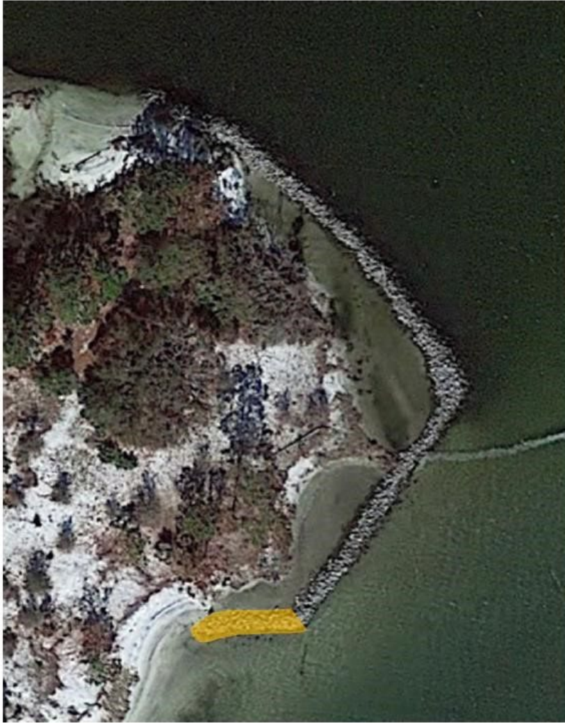
Figure 5. The yellow polygon indicates the segment of the Robinson Island revetment that will not be modified during project construction.
