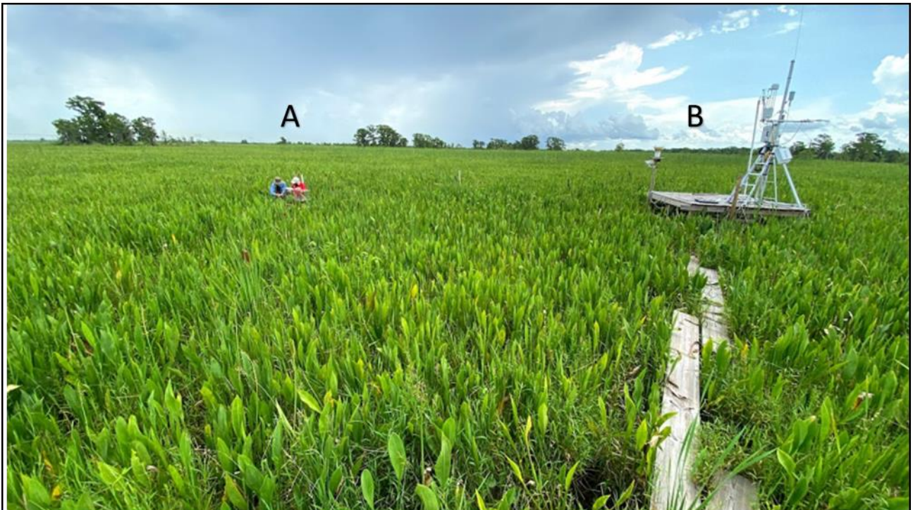
Figure 5. Vertical flux station located in the fresh marsh. Vertical greenhouse gas data collection from A) chambers and B) eddy covariance tower.
