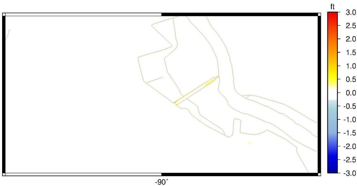
Figure 4-2. Change in Peak Wave Heights During 1 Percent AEP Storm (Storm 009): 2070 Applicant's Preferred Alternative + Open Conveyance Channel Less 2070 Applicant's Preferred Alternative.
