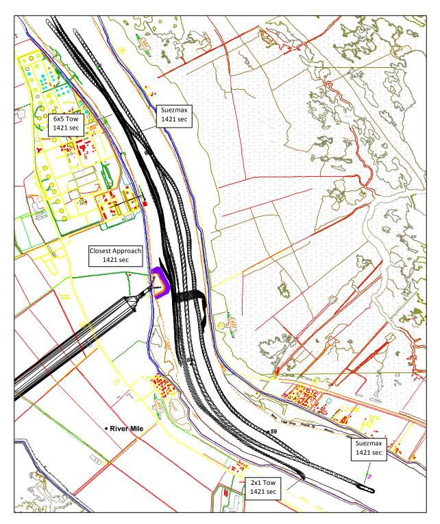
Figure A-40: Run 37, Cofferdam, 1M CFS, Wind ENE 20 Knots, 2x1 Tow Closest Approach
