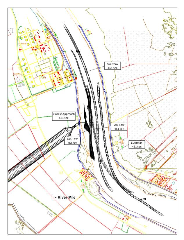
Figure A - 30: Run 48, Diversion, 1M CFS, Wind ENE 20 Knots, 4x1 Tow Closest Approach
