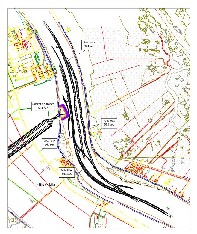
Figure A-36: Run 33, Cofferdam, 1M CFS, Wind SE 20 Knots, 2x1 Tow Closest Approach
