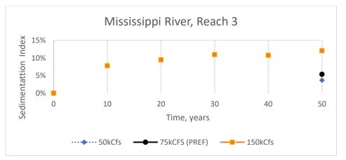
Figure 6. Basinwide Model Sedimentation Index for Reach 3 of the Mississippi River (1 Mile Below Structure) under Three Diversion Rates. Note the range of values on the y axis differs between figures.
