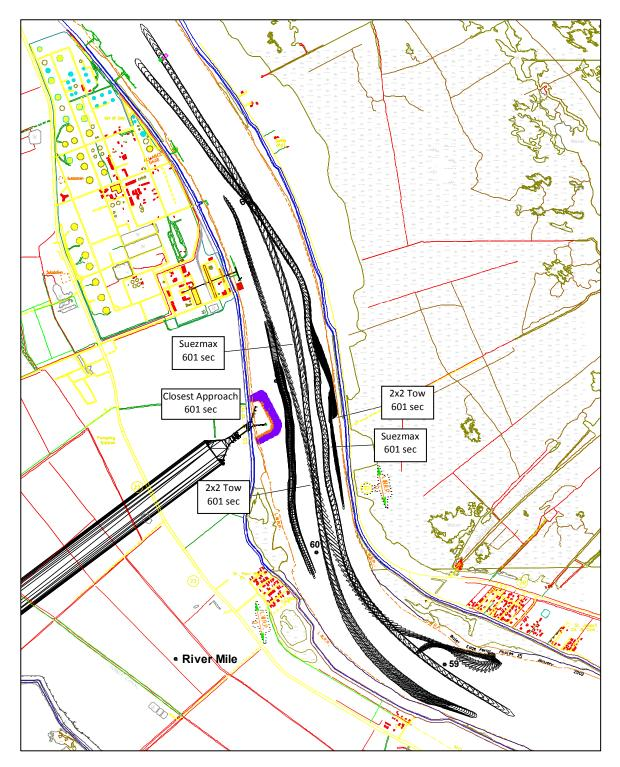
Figure A-46: Run 43, Cofferdam, 1M CFS, Wind ENE 20 Knots, 4x1 Tow Closest Approach
