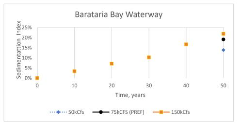
Figure 3.Delft3D Basinwide Model Sedimentation Index for the Barataria Bay Waterway<br/>under Three Diversion Rates. Note the range of values on the y axis differs<br/>between figures.
