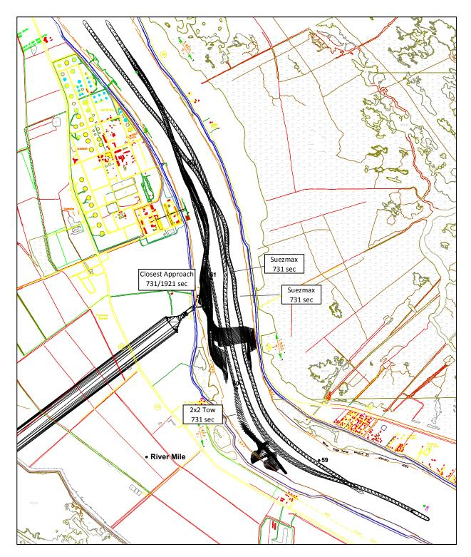
Figure A -28: Run 28, Diversion, 1M CFS, Wind ENE 20 Knots, 4x1 Tow Closest Approach
