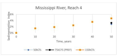
Figure 7.Delft3D Basinwide Model Sedimentation Index for Reach 4 of the Mississippi<br/>River (From 1 Mile Below Structure to Gulf) under Three Diversion Rates. Note<br/>the range of values on the y axis differs between figures.
