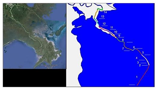
Figure 8.Map of Numbered Control Volumes used for Near- and Far-field Bed Elevation<br/>Change Analysis. This is Figure 5.9 from Brown et al. (2018 draft).
