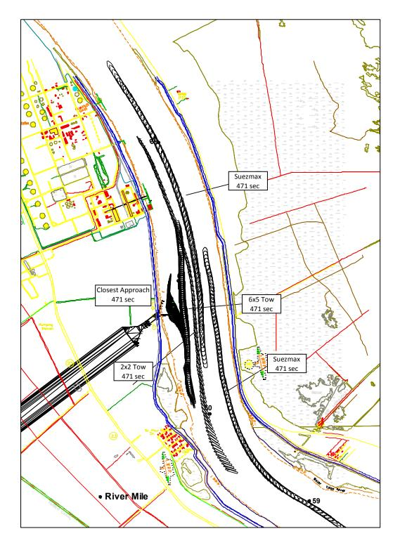
Figure A - 31: Run 49, Diversion, 1M CFS, Wind ENE 20 Knots, 4x1 Tow Closest Approach
