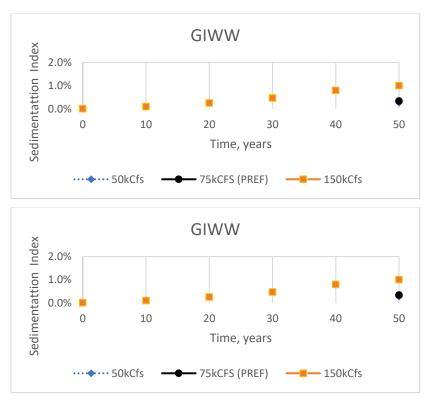
Figure 2.Delft3D Basinwide Model Sedimentation Index for the GIWW under Three<br/>Diversion Rates. Note the range of values on the y axis differs between figures.
