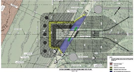
Figure 5. Proposed Construction Layout for the Mid-Barataria Sediment Diversion
