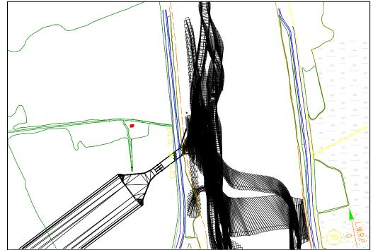
Figure 26: Composite Trackline of Tows Passing Close to Operating Diversion Pilots Noting Effect on Tow of Operating Diversion, Closest Approach <300 ft 1,000,000 cfs River Flow, SE or ENE 20-knot Wind
