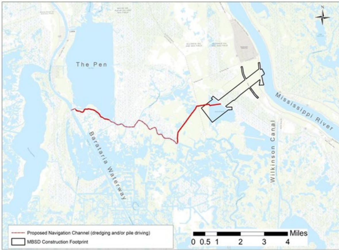
Figure 2. Planned access route from the northeast to the proposed outfall construction area (Figure 2.3.1-1 in Project BA)
