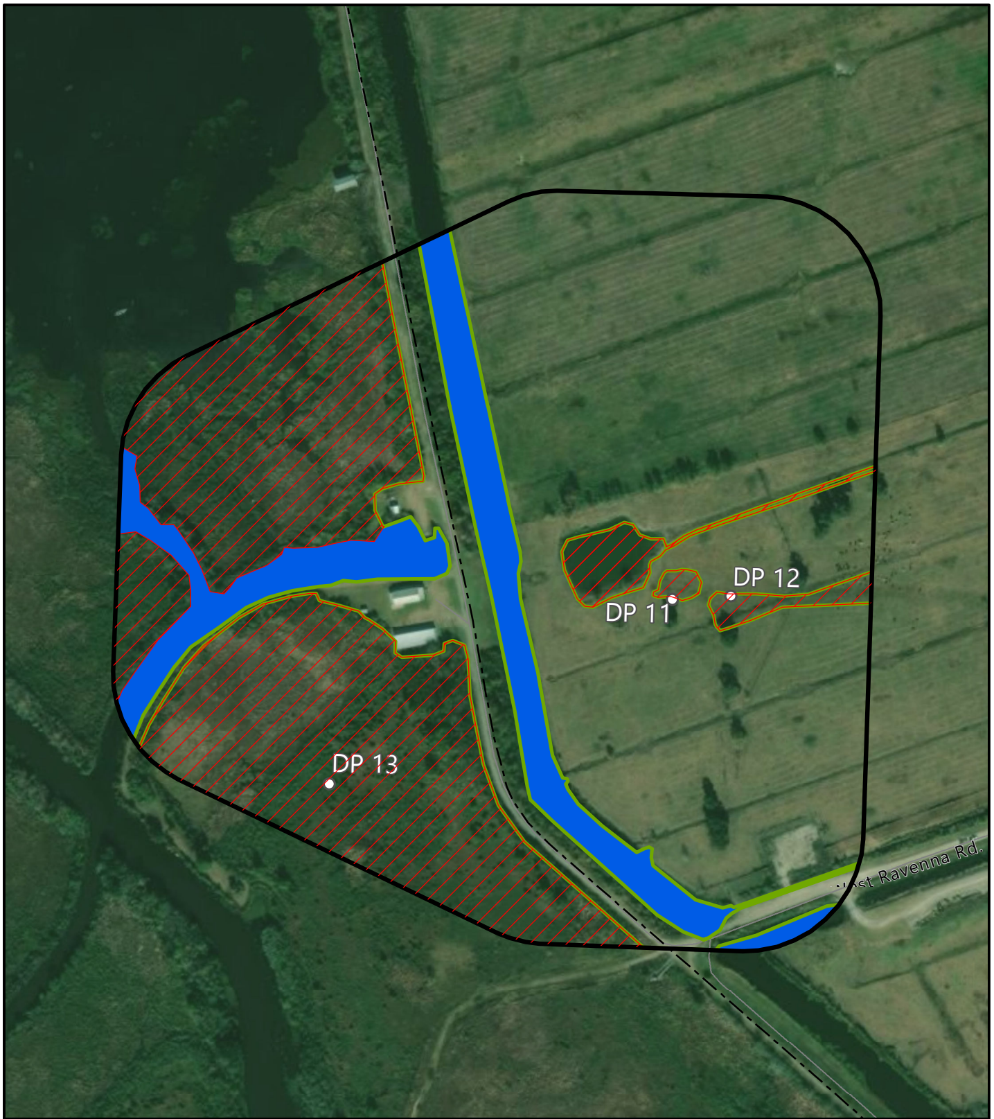
Figure 4: Wetland Delineation: Site 1, Pump Station Proposed MBSD Project, Plaquemines Parish, LA
