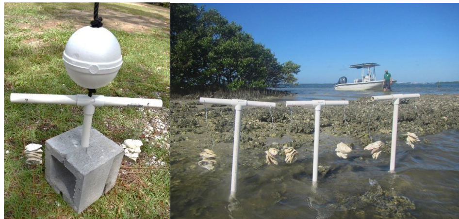
Figure 4: Subtidal (left) and intertidal (right) oyster spat traps with stringers.
