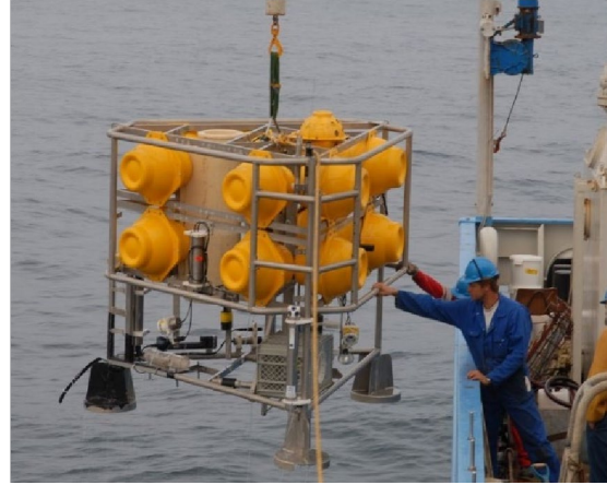
Images of a lander system. Left: this particular lander is outfitted with penetrating sediment samplers, amongst other sensors on the bottom bar; right: instrumented with camera systems and baited traps, demonstrating the flexibility of the system to achieve multiple data streams.
