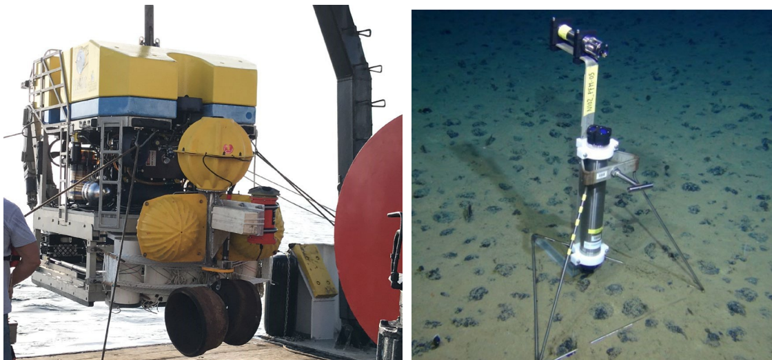
Images of the short-term lander systems. Left: bottom lander with orange acoustic Doppler current profiler and sensor under the syntactic foam floatation. Right: micro-lander system with optical fluorometry and turbidity sensor (top) and short-range acoustic Doppler current profiler.
