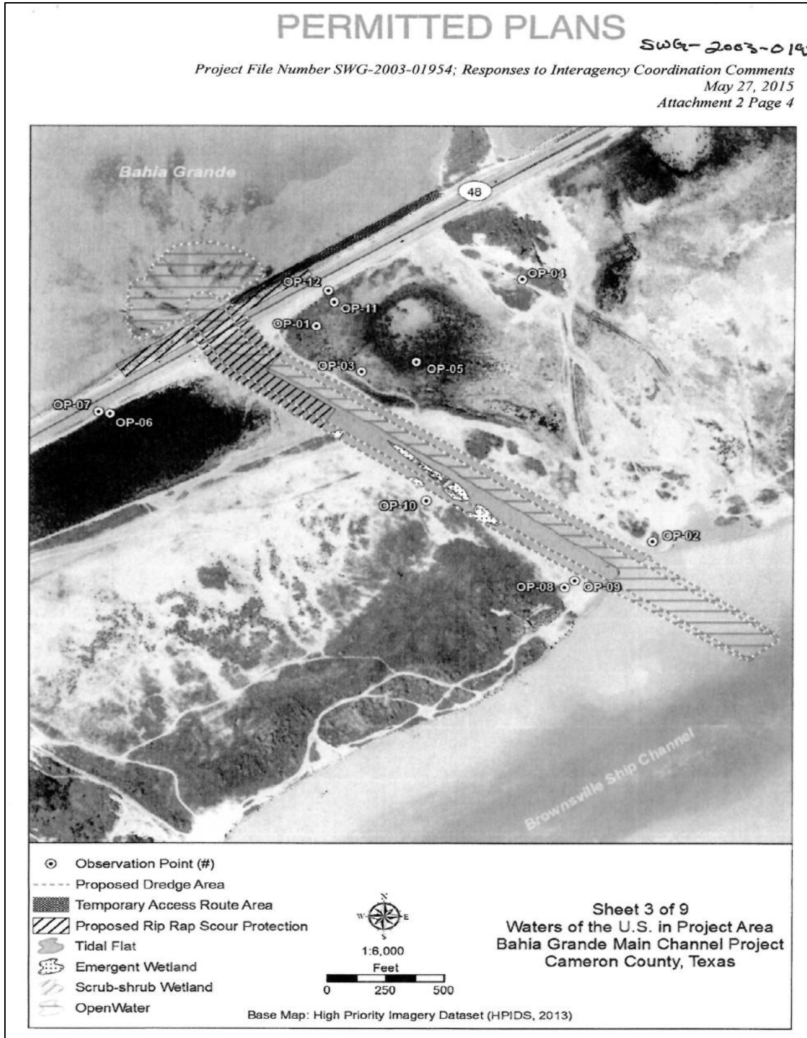
Figure 1. Aerial photo of project area showing project elements and current habitat types (Figure 2 in TPWD's Biological Evaluation Form for the Bahia Grande Hydrologic Restoration Project).
