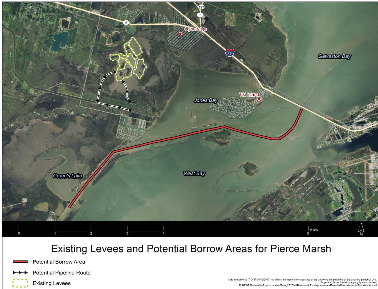
Figure 2. Location of the potential restoration areas, bounded by existing levees. Beyond the existing levees, the nearshore areas may also be restored with beneficial use of dredged material.
